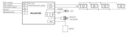
Take care that the LED is connected with the right polarity. LEDs that are connected to the EM powerLED devices should have a reverse polarity protection device such as a schottky diode fitted, otherwise irreversible damage could occur if the LED is connected in reverse polarity. Any protection device must be capaple of handling in excess of 600 mA.
