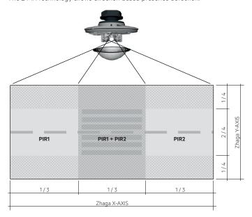
The 2 PIR technology allows direction based presence detection.
