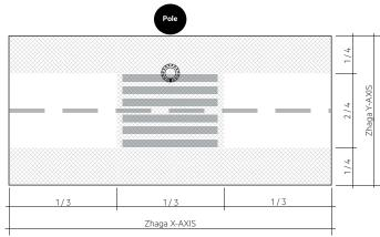
The full detection area is rectangular, the highlighted area is optimized for detection of pedestrians. The detection area is not sharp-edged but runs smoothly over the marked borders.
